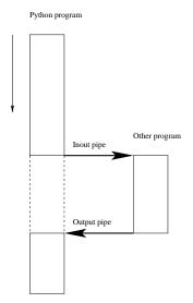
A simple example is to let Python call up the standard UNIX command wc -w (word count), supply some input through the input pipe and retrieve the result through the output pipe. The command is used to count the number of words in the input string<sup>2</sup>. First we need to open the pipes:
