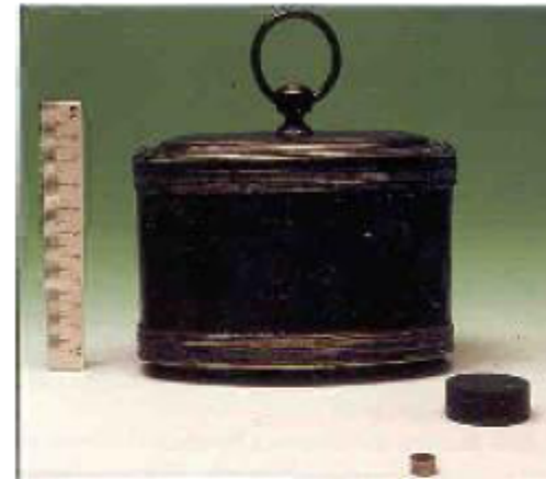
A lodestone magnet from the 1750's and typical ferrite and rare earth used in modern appliances. Each of these contain about 1J of magnetic energy.
