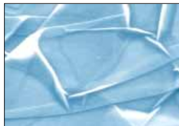
Scanning electron micrograph of a strongly crumpled graphene sheet on a silicon wafer (Foundation of Fundamental Research on Matter, the Netherlands).
