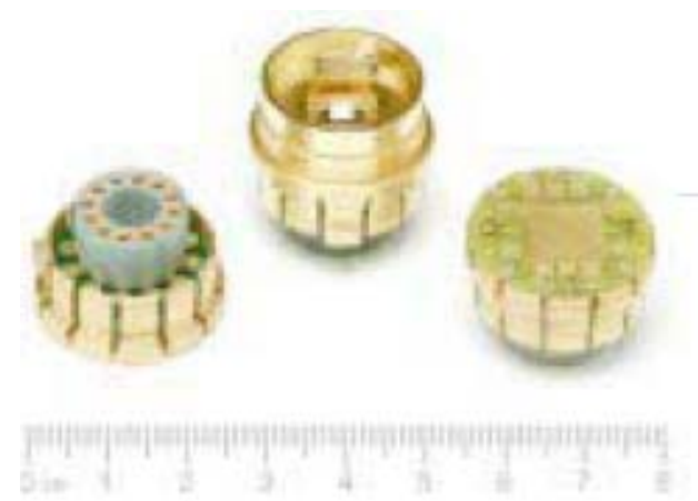
► Specialized pucks, 2.4 cm in diameter, are used for different measurement applications.
